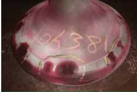
1 Worn/burned seating area
