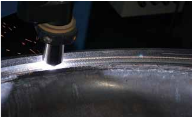
3 MIG welding St.St. O-ring grooves/base layer Plasma welding seating layer Stellite/ hardfacing
