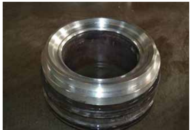
2 Premachining of seating area and O-ring grooves
