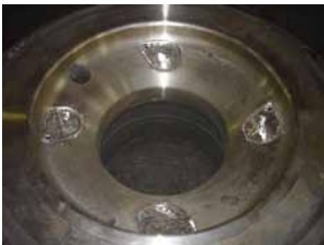
7 Inconel welding/ grinding radius
