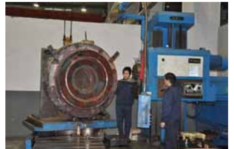
6 Redrilling of all pockets and cooling bores
