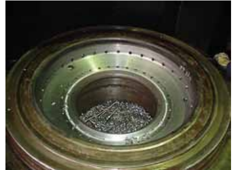
3 Premachining/check by MPI to ensure crack free
