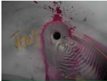
2 Cleaning/inspection incl MPI/dye check
