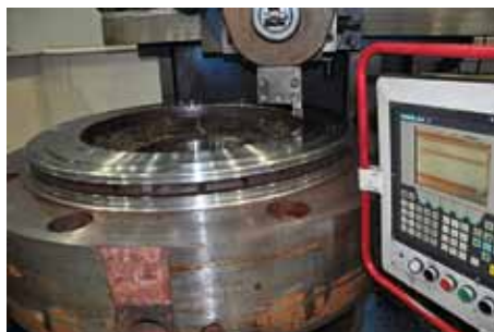
8 CNC machining to original dimension
